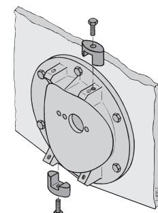
Install de thrust tunnel onto the flange with the supplied bolts en washers.
