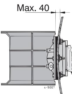
In case that the available height at the stern is insufficient for the installation of the stern thruster a sloped surface can be made to install the stern thruster. Than keep in mind that the thrust tunnel must be protected against the forces caused by the water flow during normal cruising.
