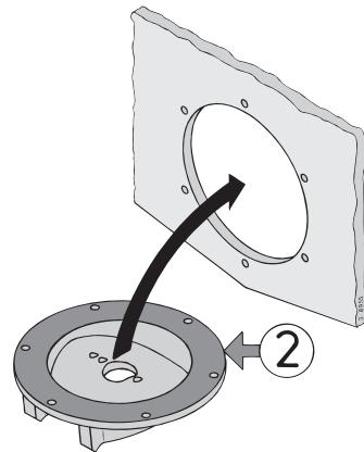
Install the flange with the supplied bolts, nuts and washers.
